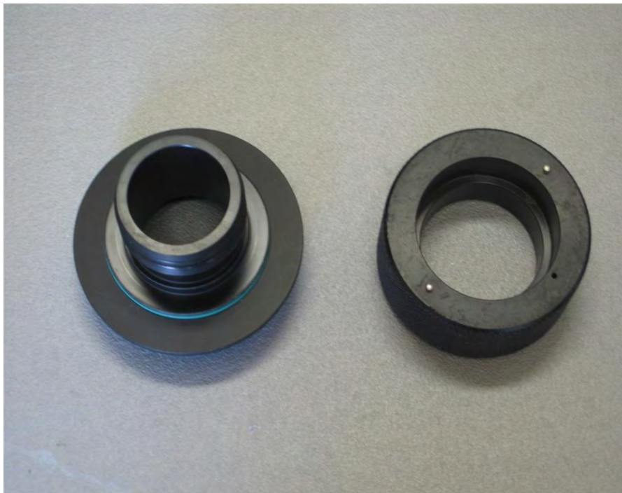
Top of sensor chamber and assembly tool
