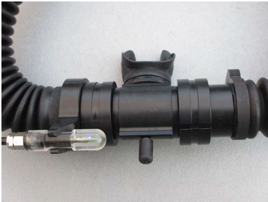
Open mouthpiece (the lever shows to the front and forwards)
