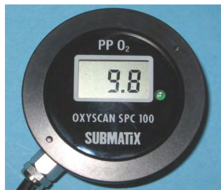
display of mVolt of sensor (example: 9.8 mV)
