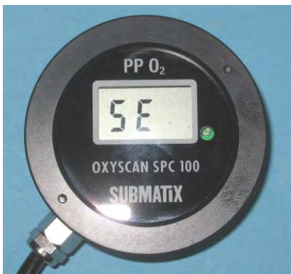
„SE“ (sensor exists): sensor Is connected
