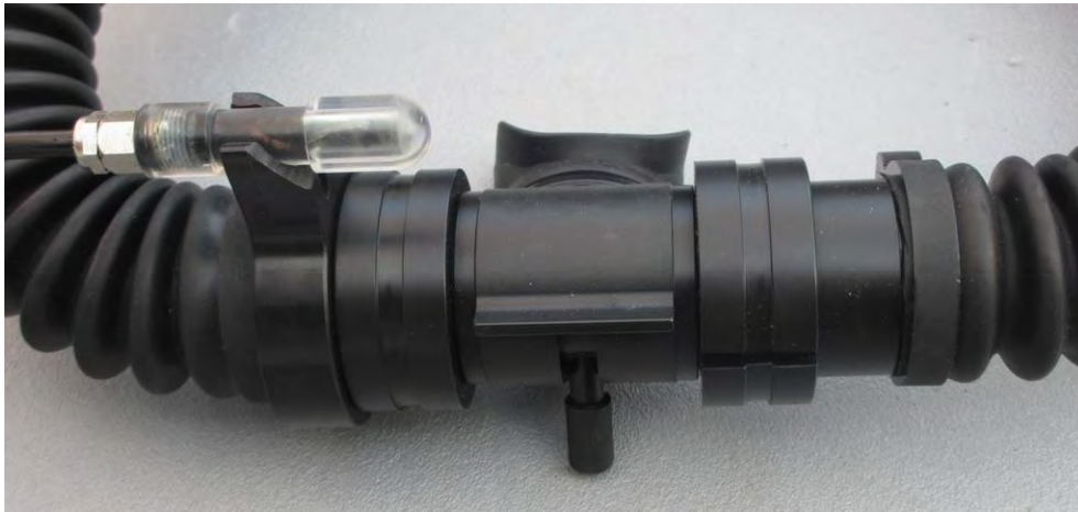
Closed mouthpiece (the lever points down)
